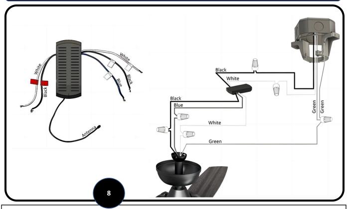
**8.** Use the supplied wire connectors to connect the fan wires to the remote receiver and then the receiver to the power supply wires according to the wiring diagram and following instructions:
