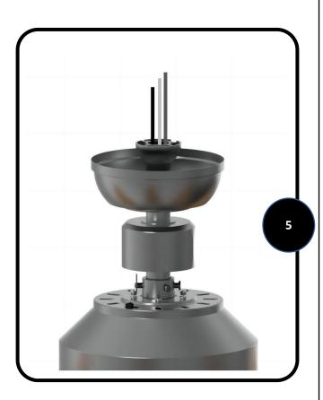
Loosen but do not remove the two set screws in the yoke. Set screws need to be loosened enough to fully insert the downrod.
