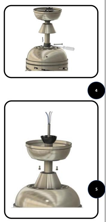
Loosen but do not remove the two set screws in the yoke. Set screws need to be loosened enough to fully insert the downrod.
