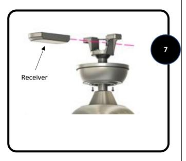
Lift the downrod into the mounting bracket. Rotate the downrod until the tab in the mounting bracket is seated in the slot in the downrod ball.
