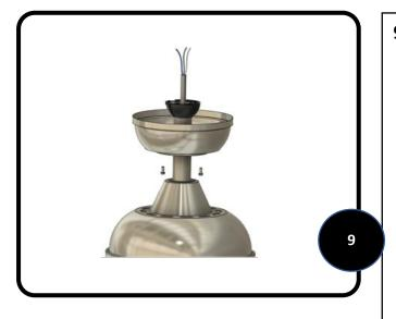
9. Locate the (2) screws on underside of hanging bracket and loosen screws. Place rounded part of slotted hole in canopy over the loosened screws in hanging bracket and push up. Make sure all wires are tucked into the canopy and will not be pinched, including the black antenna wire. Twist canopy to lock. Tighten screws securely.
