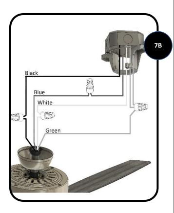
Use the supplied wire connectors to connect the fan wires to the power supply wires according to the wiring diagram and following instructions:
