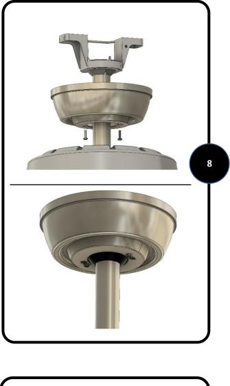
Locate the (2) screws on the underside of hanging bracket and loosen screws. Place rounded part of slotted hole in canopy over the loosened screws in hanging bracket and push up. Twist canopy to lock. Tighten screws securely.
