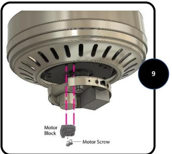
**9.** Remove the five motor blocks and five motor screws from the underside of the motor. Discard the motor blocks but keep the motor screws for installation of the blade arms.
