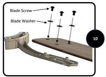
along with the blade washers, through the blade and into the blade arm, tighten each screw blade screw, starting with the one in the middle. Repeat this step for the remaining blades and blade arms.
