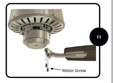
11. Secure the blade arm to the underside of the motor using the motor screws removed in Step 10. Secure each blade arm to motor before moving to the next.
