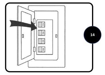
**14.**Restore the power to the main fuse or circuit breaker.
