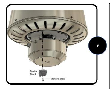
9. Remove the five motor blocks and five motor screws from the underside of the motor. Discard the motor blocks but keep the motor screws for installation of the blade arms.
