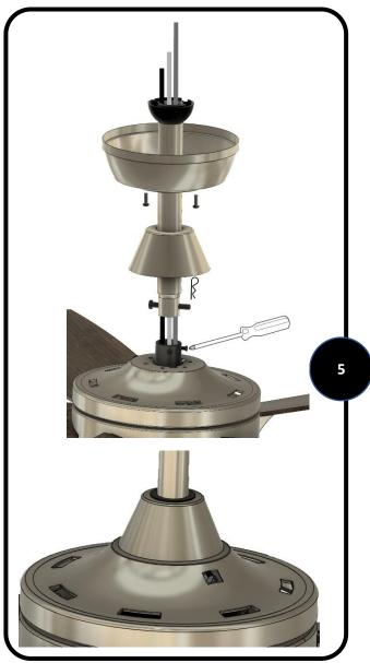
Loosen but do not remove the two set screws in the yoke. Set screws need to be loosened enough to fully insert the downrod.
