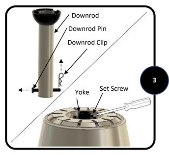
3. DOWNROD MOUNT – Remove the downrod pin and downrod clip from the downrod. Then loosen but do not remove the two set screws in the yoke. Set screws need to be loosened enough to fully insert the downrod.
