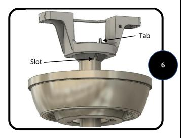
**6.** Lift the downrod into the mounting bracket. Rotate the downrod until the tab in the mounting bracket is seated in the slot in the downrod ball.
