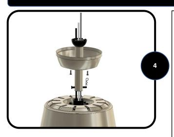
**4.** Feed the wires coming from the yoke through the canopy and downrod.
