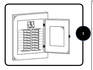
**1.** Turn OFF the electrical power at the main fuse or circuit breakers.
