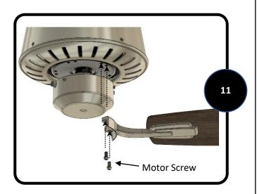
**9.** Remove the five motor blocks and five motor screws from the underside of the motor. Discard the motor blocks but keep the motor screws for installation of the blade arms.
